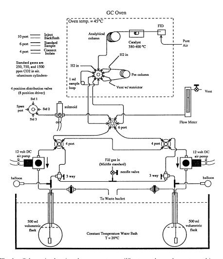
**Fig. 1** Schematic showing the gas—water equilibrator and gas chromatographic system for the equilibration of  $p(CO_2)$  in discrete samples (Chipman *et al.*, 1992).
