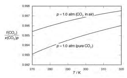
**Fig. 1** Variation of the fugacity coefficient with temperature at 1 atm total pressure for pure  $CO_2$  gas and for  $CO_2$  in air:  $x(CO_2) = 350 \times 10^{-6}$  (calculated using the procedure described in SOP 24 of this Guide).
