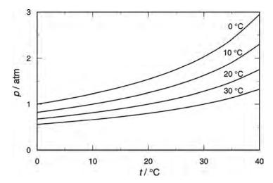
**Fig. 1** Pressure in headspace with r = 0.01 as a function of temperature for various initial temperatures. In calculating this, it was assumed that the gases— $N_2$ ,  $O_2$ ,  $A_1$ ,  $O_2$ —were initially at solubility equilibrium with sea water at the starting temperature, that they behaved ideally and that the initial pressure in the bottle at the indicated temperature was 1 atm.
