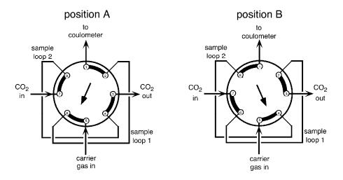
**Fig. 1** Plumbing of a gas loop calibration valve.
