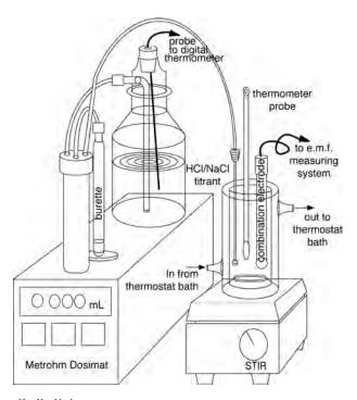
Fig. 1 Open-cell alkalinity measurement set-up.
