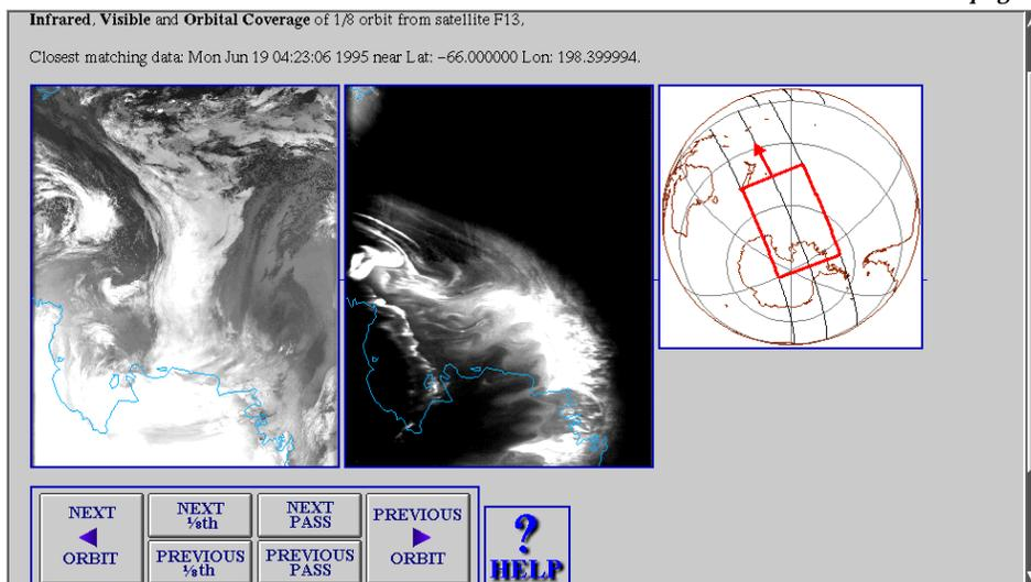
▲ Figure 3. DMSP satellites collect visible and thermal infrared imagery in global coverage along a 3000-mile swath with the Operational Linescan System (OLS.) Users within SPIDR can select DMSP imagery by date and geographical position anywhere on earth. DMSP images are then returned along with the satellite path and a button tool for navigating the database, i.e., by 'flying' the satellite about the globe.
