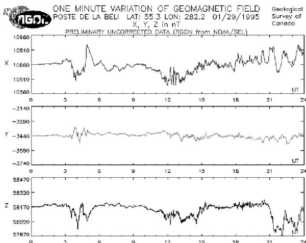
▲ Figure 6. Geomagnetic one-minute variations for 1990 through 1996 reside in a database management system. Selected data are plotted and distributed over the WWW.
