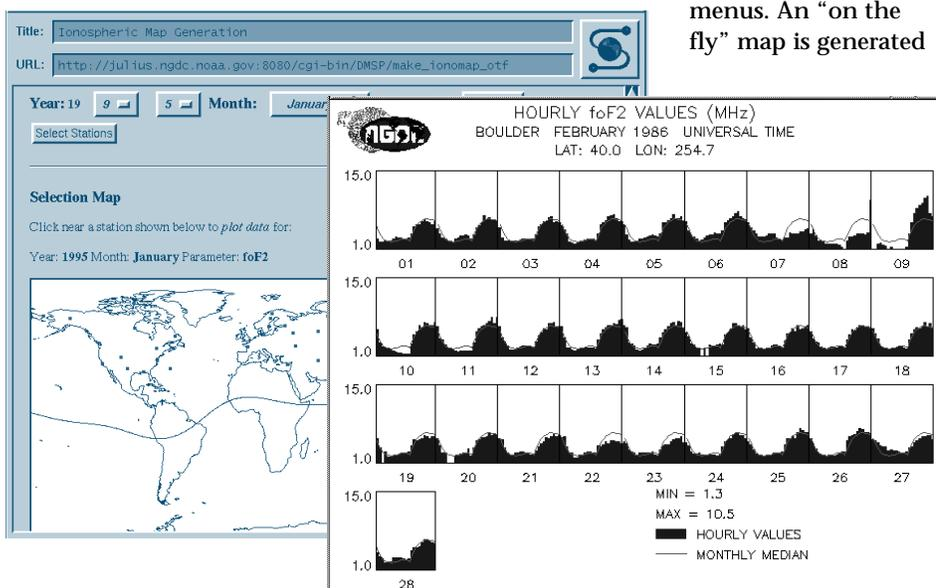
▲ Figure 5. Ionospheric maximum electron density data plot for Boulder during the February 1986 storm. The gray line indicates median values for the month. Users can select from four solar cycles of ionospheric data by global location.
