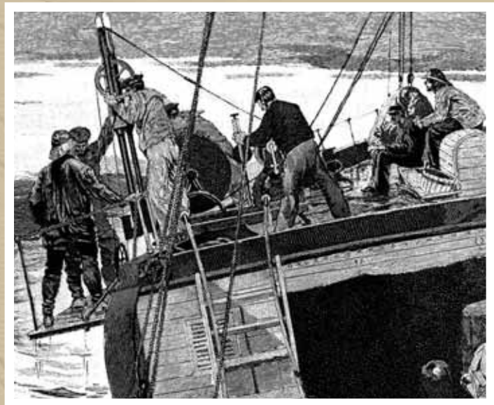
"Sounding the abyss with piano wire." This image is among the most realistic representations of sounding with the Sigsbee Sounding Machine. Most of the deep-sea soundings made prior to the advent of acoustic systems were made with piano-wire sounding machines. "The United States Fish Commission", by Richard Rathbun. Century Magazine, Vol. 43, Issue 5.1892.
