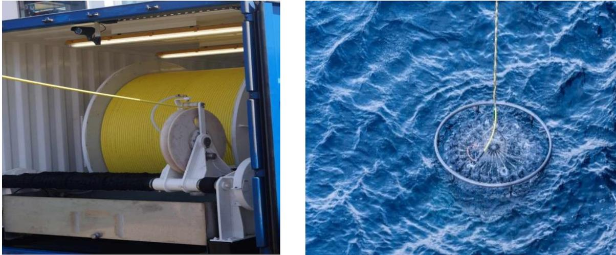
**Fig. 4.1** Left: Winch with Kevlar conducting wire. Right: Deployment of titanium CTD frame. Photo E. Achterberg (left) and C. Rohleder (right).
