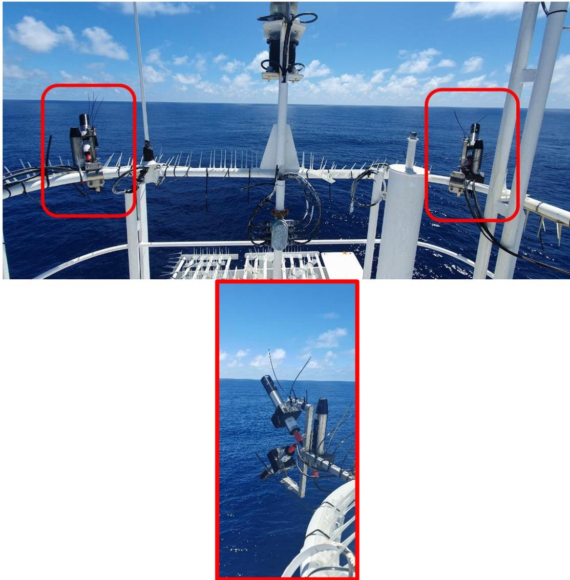
**Fig. 5.3** TriOS hyperspectral radiometers and irradiance meters on top of the mast at the bow of RV SONNE during the cruise SO298.
