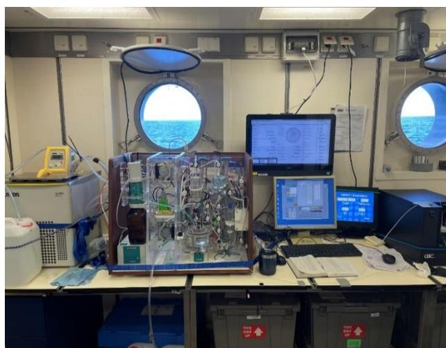
of Total dissolved inorganic carbon and Alkalinity, MARIANDA - marine analytics and data), which simultaneously measures TA by potentiometric titration and DIC by coulometric titration, with a precision < 2 µmol kg<sup>-1</sup> (Shadwick et al. 2011) respectively. A Certified Reference Material (CRM, Batch #198, #201, and #203) provided by Andrew G. Dickson (Scripps Institution of Oceanography) was used for calibration.
