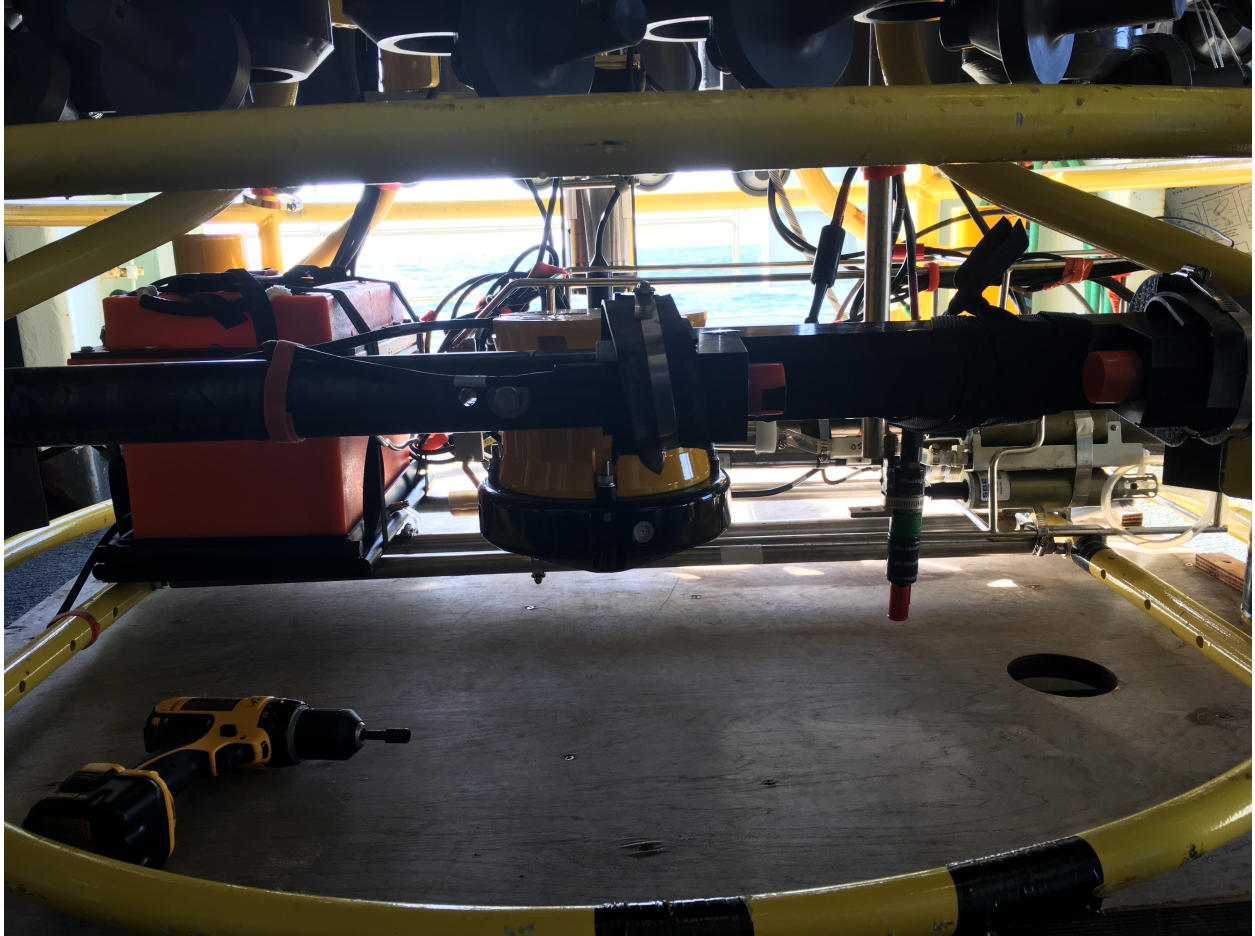
Fig. 3: Package sensor setup from left to right, LADCP battery, LADCP, transmissometer, chipod, CTD in back right.
