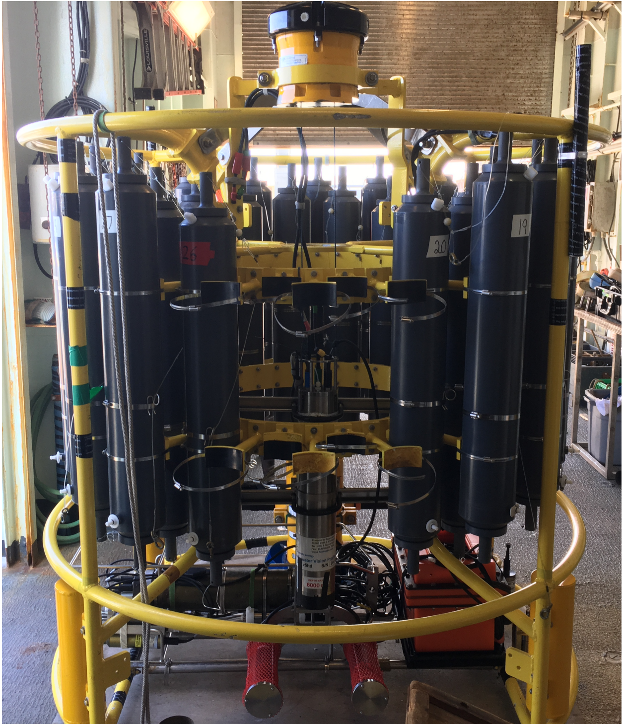
Fig. 1: Package sensor looking into the rosette from the south, with UVP directly in front of the camera.
