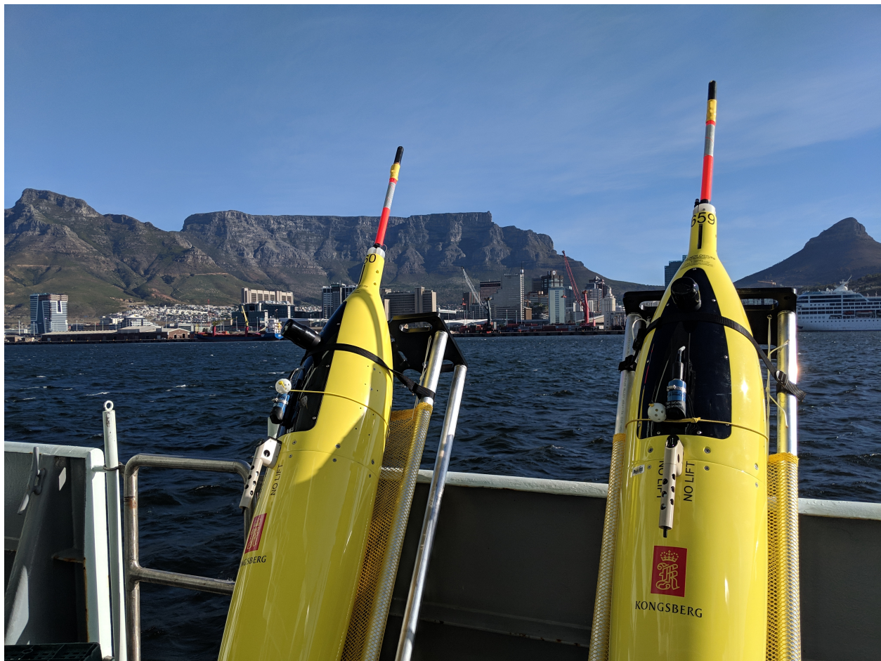
Fig. 2: Self-tests and simulation-dives were run with the gliders ratchet strapped to the back deck, in port in Cape Town (Giuliana Viglione)
