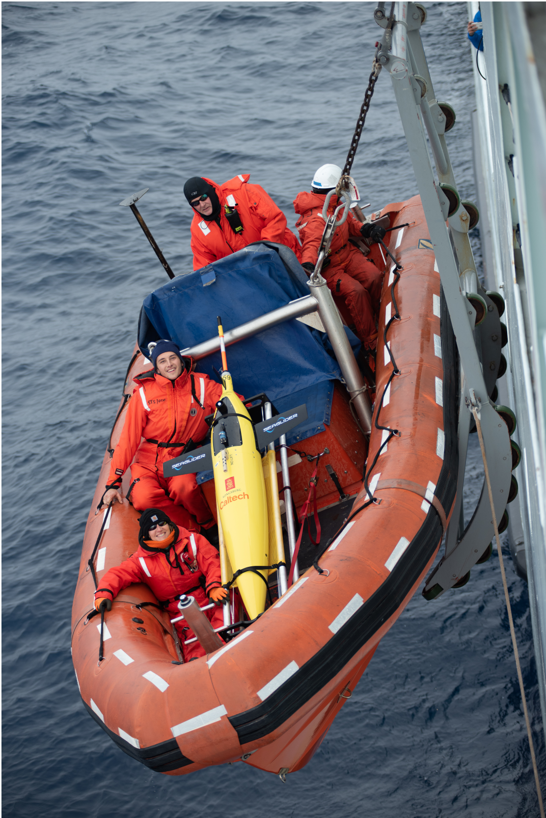
Fig. 4: zodiac lowered over side of ship with SG 660 ratchet strapped to the centre in its cradle. (Andrew Collins)
