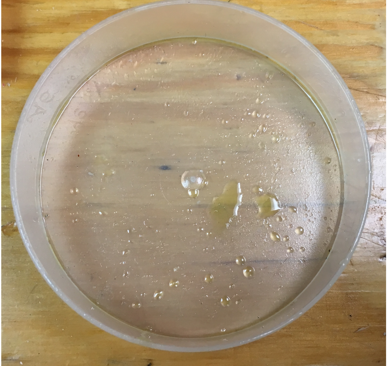
Fig. 9: Tiny amount of oil dripped out from the pressure port due to gravity. No free oil was visible to the eye in the sensor.
