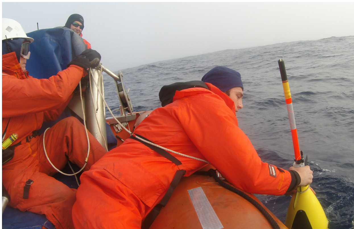
Fig. 6: SG 660 is held in the water until the rudder and antenna are above the water line. (Isa Rosso)
