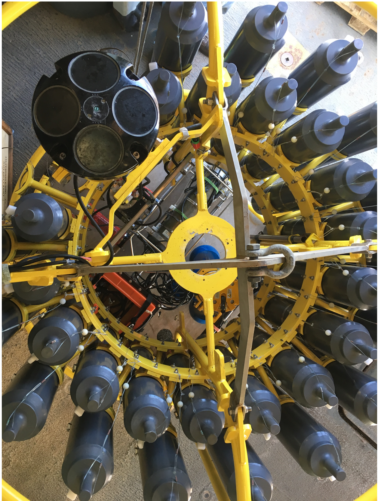
Fig. 2: Package sensor setup with top as southeast, to show in order from top clockwards CTD, downward LADCP, LADCP battery, and UVP.
