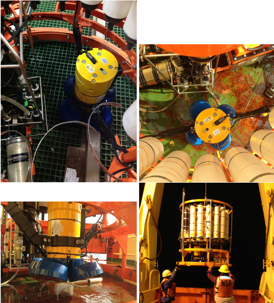
Figure 12: The WH150 mounted in the rosette. Upper left: along the left from bottom to top are the IMP, the CTD, and (barely visible) the SOB. Upper right: view from above. The IMP, CTD, and SOB are visible along the top. Lower left: view of the clamp. Note the mark showing beam 3. Lower right: the rosette at launch shows vertical positions more clearly. The spar on the left has a \chi -pod thermistor at the top and a \chi -pod data acquisition module hose-clamped to it.
