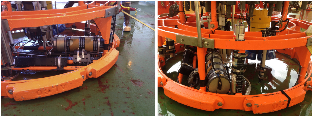
Figure 15: The IMP in the rosette. The photo on the left also shows the transmissometer, fluorometer, and CTD cage. Behind the CTD is the WH150 and behind the IMP is the down-facing \chi -pod thermistor and (mostly hidden,) a \chi -pod acquisition module. At far lower left, the clamps holding the altimeter are visible. In the right photo, the \chi -pod components are more visible, as are the altimeter and WH150.
