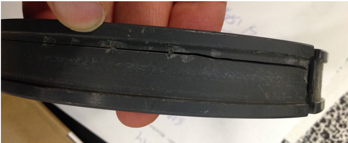
Figure 2: The broken band clamp from the first station.
