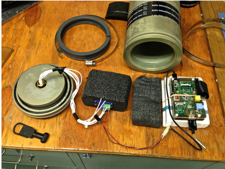
Figure 14: The IMP, disassembled. The Raspberry Pi is on the right, with the USB WiFi dongle at the bottom. The sensor board is in the styrofoam box rubber-banded to the Pi. That was shoved to the far end of the pressure vessel (top), followed by the foam pad and then the DC/DC converter encased in foam. Note the precision voltage regulator between the DC/DC converter and the Pi. The DC/DC converter was powered through pins 3 (+) and 7 (-) of the male Impulse bulkhead connector in the end cap.
