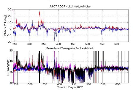
the reported BT Range is not the slant range along the beam (37m/cos(20deg)=39m), but has been corrected nominally by the instrument beam angle as per the email from RDI.
