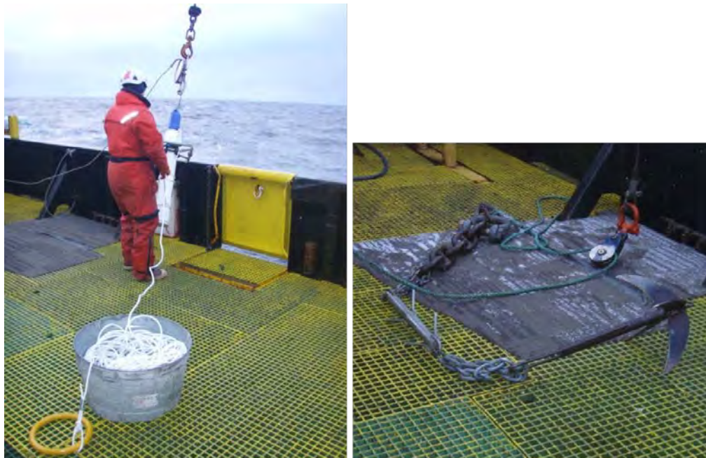
Figure 3. (Left) An Autonomous Underwater Recorder for Acoustic Listening, Model 2 (AURAL) ready for deployment from the Norseman II in summer 2012 in the northeastern Chukchi Sea. (Right) Grapple recovery gear ready for use on the Norseman II .
