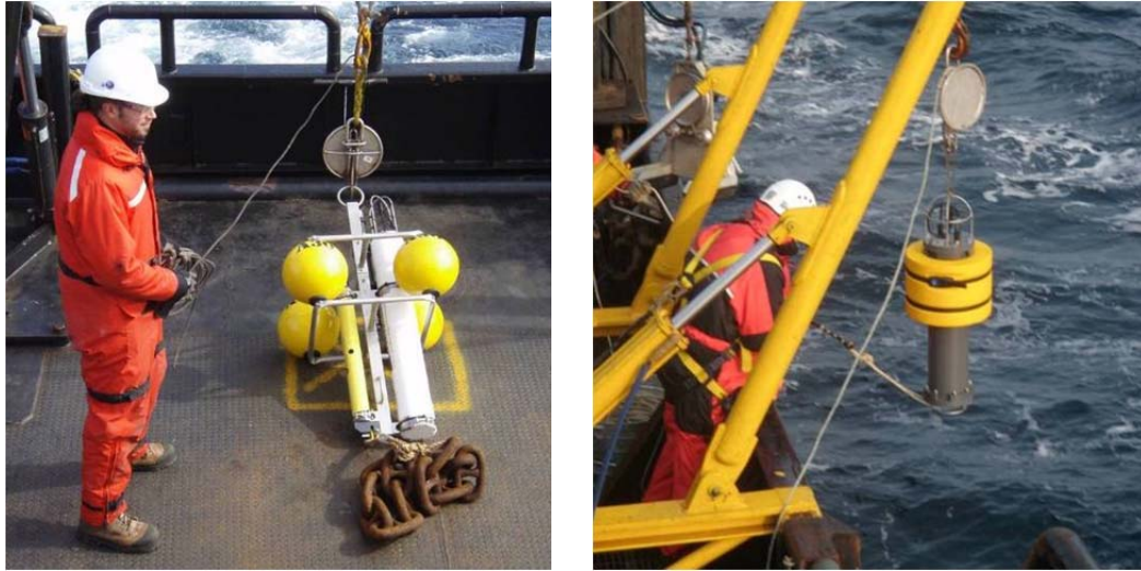
Figure 1. AURAL Recorder ready for deployment (left) and AMAR deployment from the Westward Wind during the summer 2009 in the Alaskan Chukchi Sea (right).
