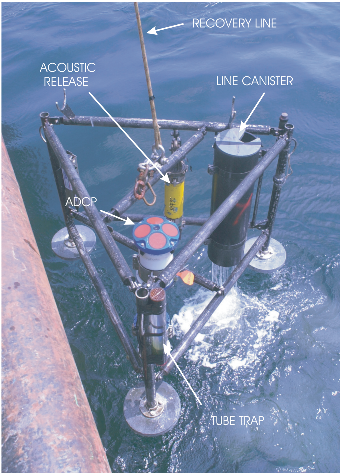
Figure 7B. A micropod being recovered. The upward-looking Acoustic Doppler Current Profiler (ADCP), mounted in a corner of the triangular frame, has two pairs of transducers that measure currents in orthogonal directions. The rope canister contains line (in this picture the canister is empty) that is pulled to the surface by a float released by the acoustic release.
