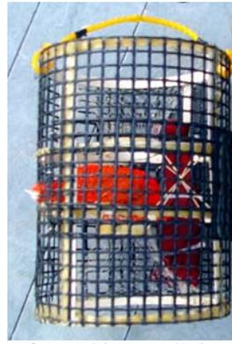
Figure 6 Benthic trap designed to fit in BioBox
