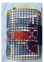
Figure 6 Benthic trap designed to fit in BioBox
