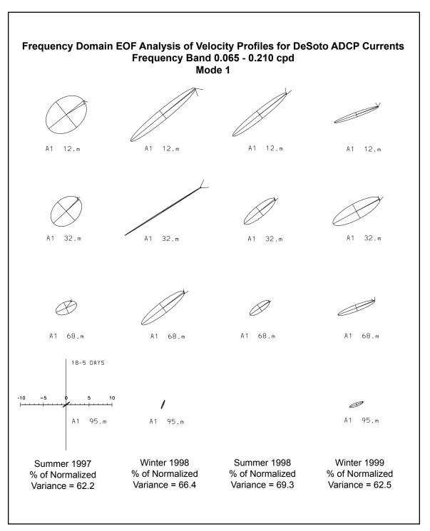
Figure 6.2-7a. Results of FEOF analyis for mode 1 at mooring A1 for summer and winter seasons presented as ellipses for selected depths. The length of the major/minor axes represent the amplitudes of the mode for the v and u current components. The arrow gives the relative phase of the mode.
