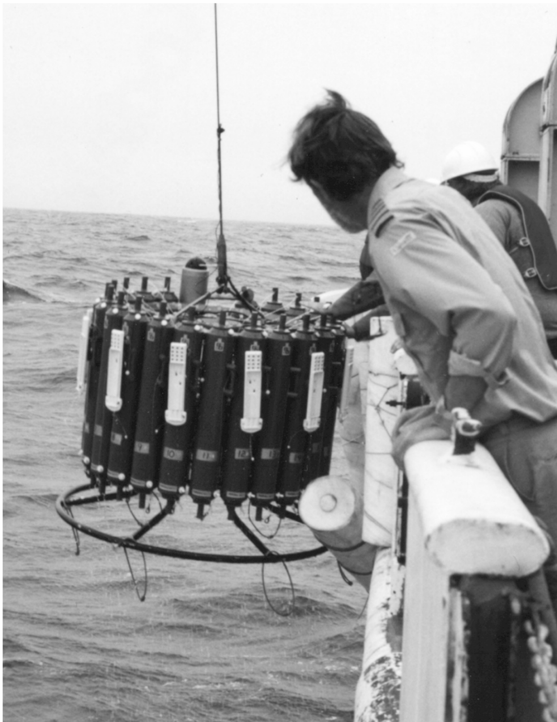
General Oceanics Rosette showing 10 litre sampling bottles
