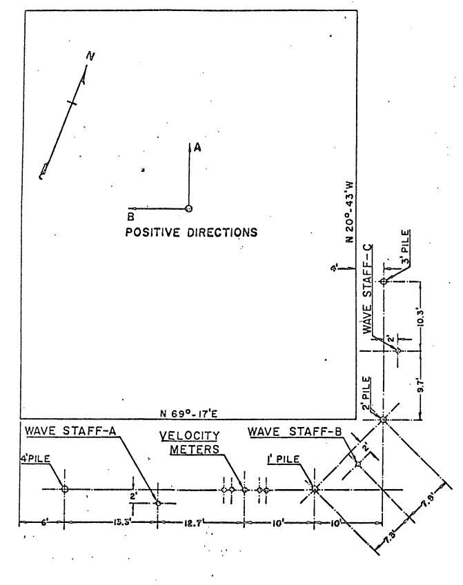
FIGURE I PLAN VIEW OF TEST UNITS (AFTER AUGUST 1956)
