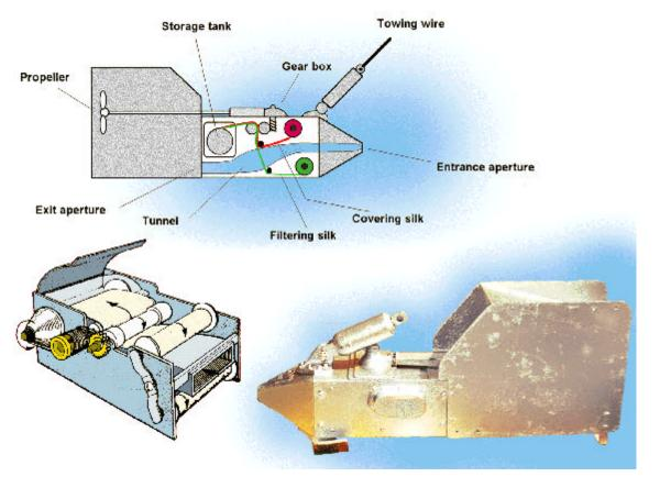
Diagram showing a cutaway vie of the CPR the plankto filtering mechanism and a photograph of the instrument
