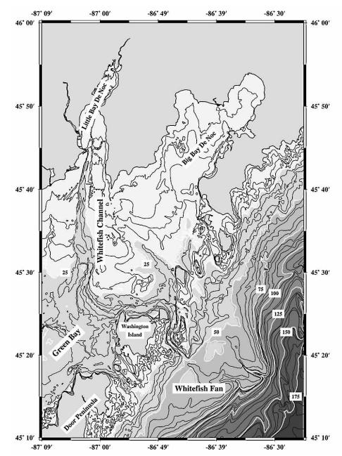
▲ Figure 2. New bathymetry of the Whitefish Fan and Channel, Lake Michigan. Contour interval is five meters.
