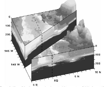
▲ Figure 3. View of the three-dimensional equatorial temperature field in August 1992, looking towards the northwest. The equator is represented by a dashed line. This data plot was produced from JGOFS cruise data by Michael Sawyer, June Firing and Pierre Flament of the Satellite Ocean Laboratory, University of Hawaii. The color version of the plot can be accessed through the WWW at: *http://satftp.soest.hawaii.edu/jgofs.html.*
