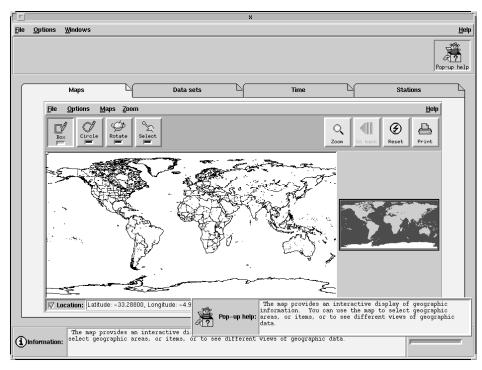
▲ Figure 4. Prototype client-server GCPS interface. The data browsing and extraction subsystem, named Xtract, is a graphical tool which utilizes the Xerox WWW/Mosaic map server to generate geographic map images. Through this main window, users may select data via a map interface as shown or by specifying particular data sets or stations.
