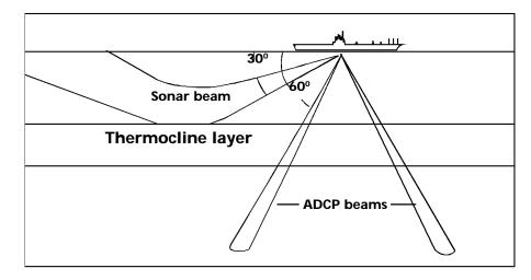
▲ Figure 1. Diagram of hull-mounted acoustic Doppler current profiler and acoustic beams utilized in developing current profiles. Three acoustic beams sent in different directions are the minimal requirement for measuring current velocity components.
