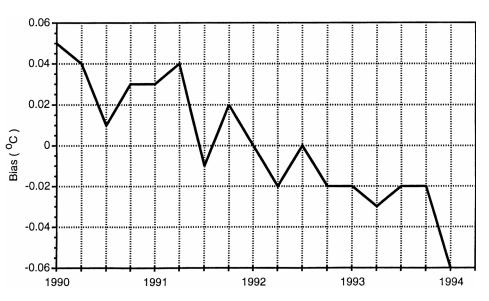
▲ **Figure 3**. MSU2R tropospheric temperature bias (plotted by year) attributed to diurnal sampling changes due to orbital satellite drift (Christy, *et al.*, 1995)
