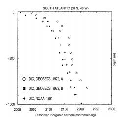
▲ Figure 2. Dissolved inorganic carbon measured in 1972 using gas chromatog-raphy (circles) and potentiometric titration (squares), and in 1991.
