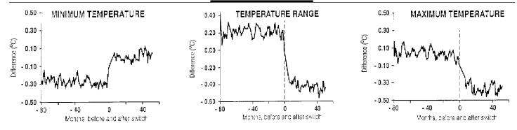
▲ Figure 1. Average differences of temperature between stations prior and subsequent to the switch from liquid-in-glass maximumminimum thermometers in a wooden Cotton Region Shelter to a thermistor in a plastic "Beehive" shelter (from Quayle *et al.*, 1991).
